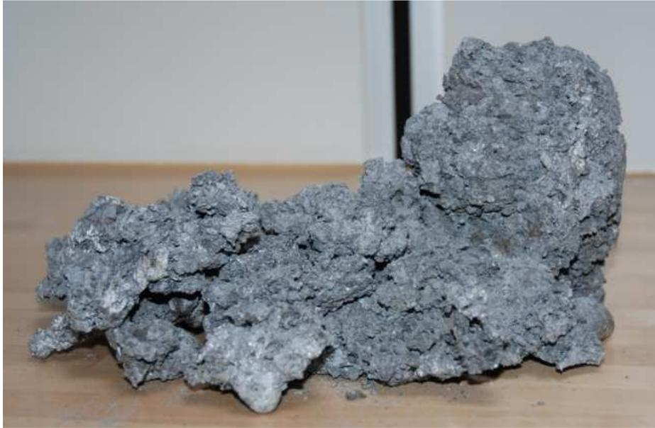
So there is a saving potential by the use of a flux, because there is more metal available for the casting process. This metal is much more worth as the costs for the flux.
