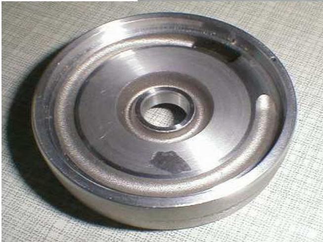
This is a high pressure die casting with a very hard inclusion. During the machining process the tooling was destroyed by this. A metallographic examination could show some corundum and agglomerates of oxides in this area.
