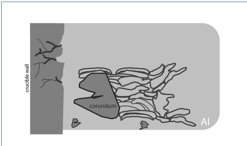
In the melt you can find some oxides, there are micro cracks in the wall. There is some sticking of the oxides at the wall, some oxides even diffuse into the micro cracks. Depending on time and temperature, some crystallization of the oxides to corundum takes place, at which the micro cracks are opened more. If the crystallization continues, some pieces of corundum can get into the melt, too.
