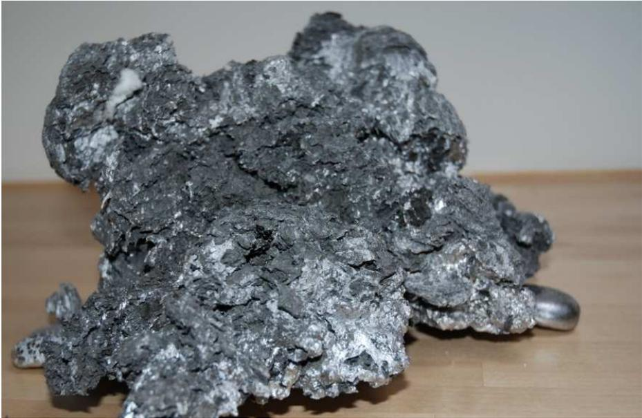
Without the use of a flux the metal content is very high, normally between 80 and 95 %. If a flux is used, the dross is fluffier, and the metal content between 20 and 35%:
